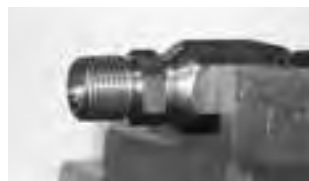
Stem properly seated against socket.
