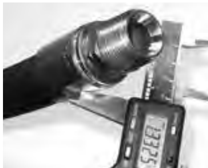
Verify crimp diameter with calipers.
