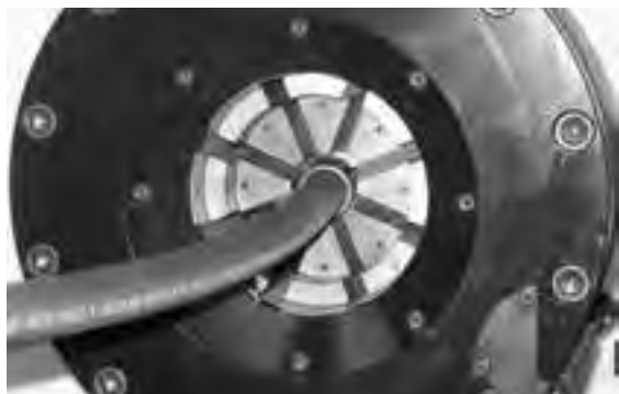
Insert hose assembly into crimper die set.
