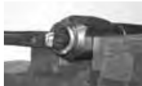
Apply lubricant to stem and hose tube.
