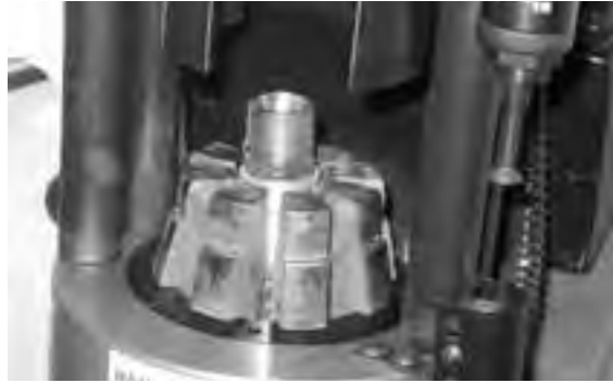
Insert hose assembly into crimper die set.
